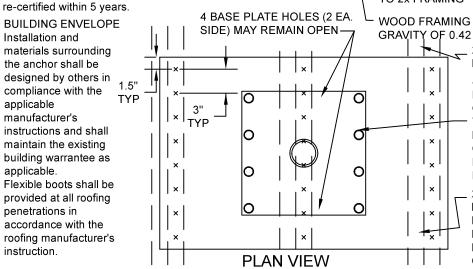
THIS DETAIL SHOP TESTS **ELASTICALLY AT 5.000 POUNDS FORCE** APPLIED AT THE TOP OF HOOP.
