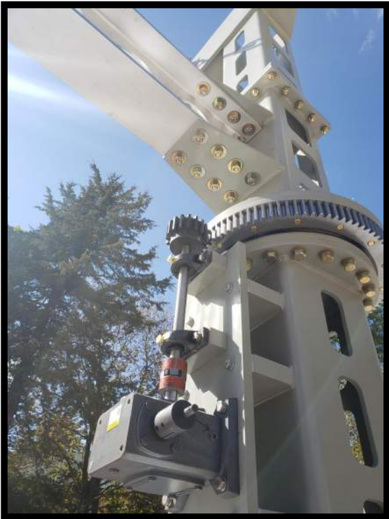
EXTRA LONG REACH DAVIT ARMS INCORPORATE POWERED DRIVES AND ARE USED FROM OVER 12'-6" REACH
