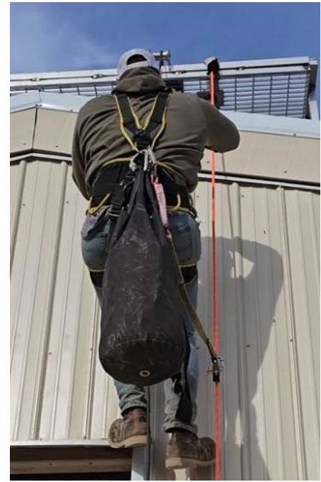
RDS USER WEIGHTED TO 310 POUNDS WITH LOAD CELL ON 1/2" STATIC KERNMANTLE ROPE
