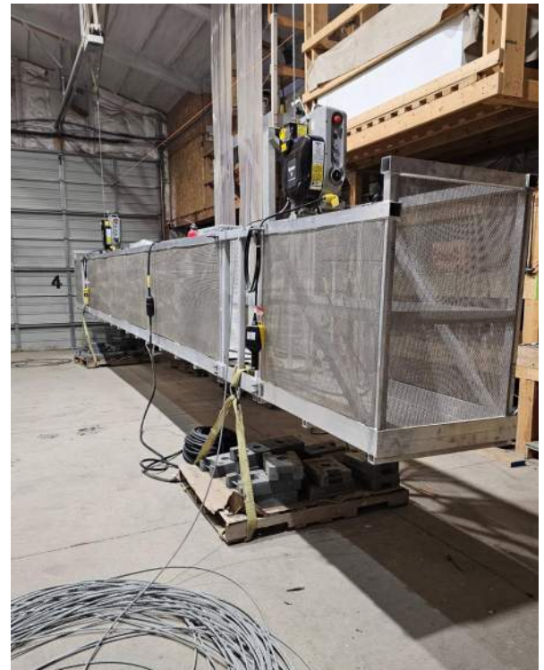
ES HOUSE STAGE UNDER FACTORY LOAD TEST WITH WIRE ROPE HOISTS THAT ES DISTRIBUTES
